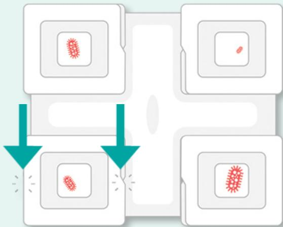
**7.** Follow instructions on the right side of this page for information on preparation of the Seal'N Freeze® Box for freezing. Place the closed Seal'N Freeze® Cryotray® with the sample inside, into the prepared Seal'N Freeze® Box by grabbing the mold at the central stud with long forceps. Please make sure the Cryotray is properly lined up with the slot in the box, and close the lid.
